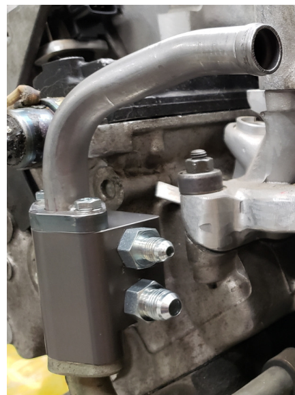
Figure 2 - Low pressure heater pipe assembled
