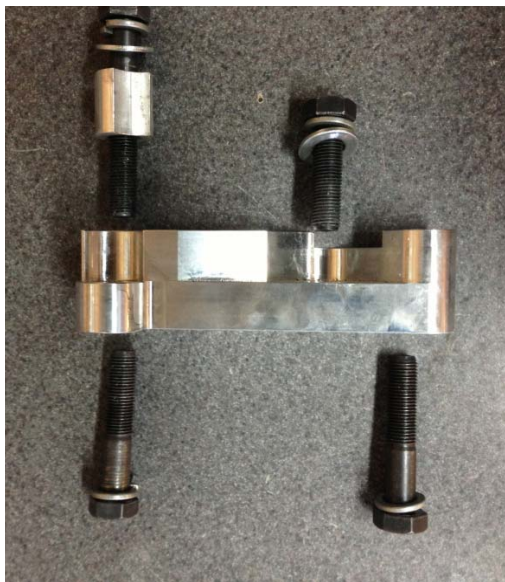
Figure 4: Bolt Assembly Order
