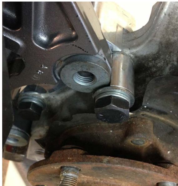
Figure 3: Slotted Washer in Position with Caliper Installed
