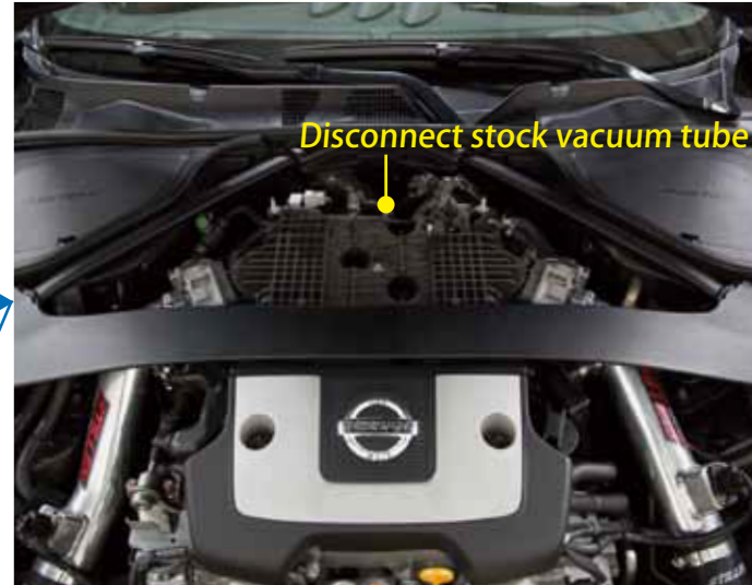
After stock vacuum tube is disconnected, re-connect it with black tube (80cm 5/16), blue silicon tube and large three-way-valves as follow
