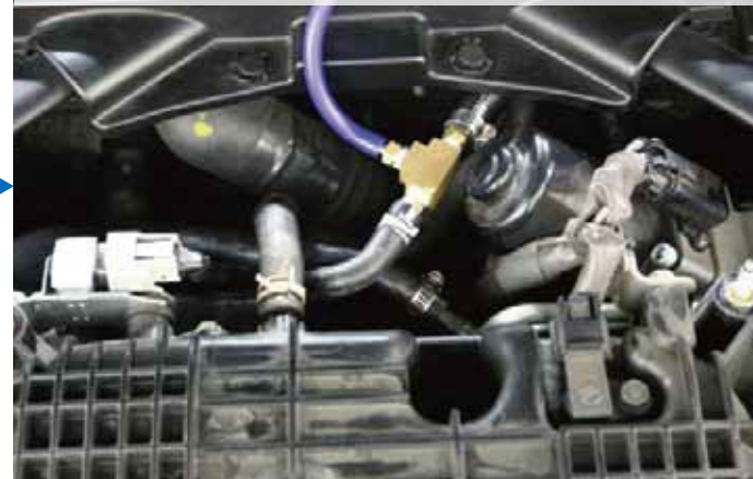
After stock vacuum tube is disconnected, re-connect it with black tube (80cm 5/16), blue silicon tube and large three-way-valves as follow
