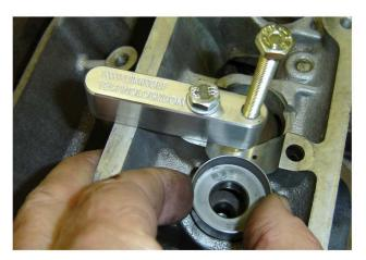
Bolt the tool to the head using the cam bearing cap bolt hole and leave it loose for now. Slide the provided bucket into the follower bore with the flat side up as shown.
