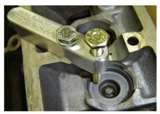
Align the tool so the compressing bolt is contacting the flat surface in the bucket and tighten the tool to the head.
