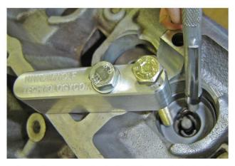
Lower the compressing bolt until it contacts the bucket, then rotate it 5 more rotations. Stop if any binding is felt and investigate! Remove the spring retainer keepers and back off the compressing tool. Loosen and rotate the tool out of the way. Remove the bucket and the spring. Assemble with the new spring in the reverse order.
