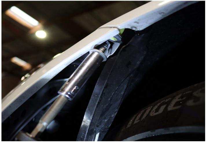
Gently detach the front bumper by pulling outward from the side, disengaging it from the mounting clips.
