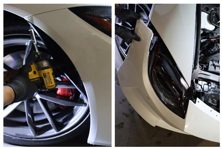
To detach the entire bumper, uninstall the ten 10mm bolts located beneath the front bumper securely.
