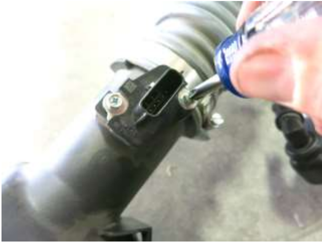
h. Remove the MAF sensors from the factory air boxes. The screws will be reused in step 3a.
