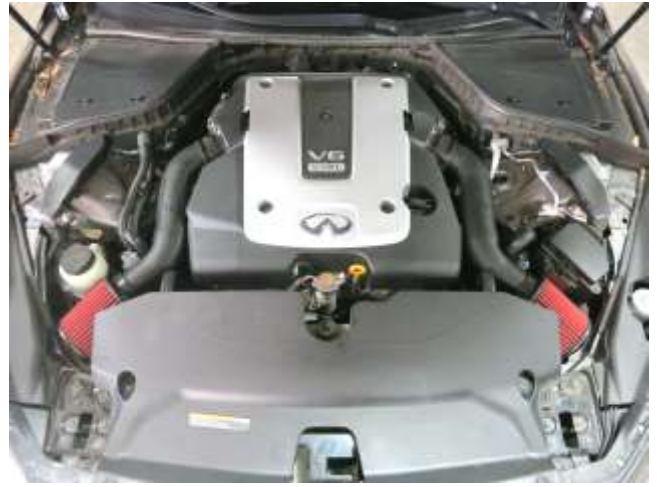
AEM INTAKE INSTALLED
