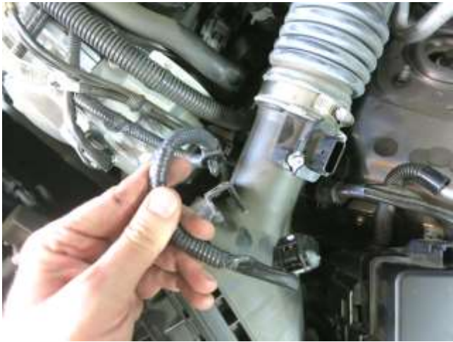
f. Disconnect the Mass Air Flow (MAF) sensor harness and remove the clip from the air box as shown on both air boxes.
