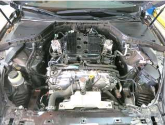
g. Remove both air box and intake hose assemblies by lifting them up and out of the engine bay. Note: Do not discard your stock equipment.
