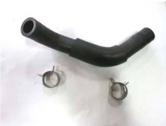
i. Remove the stock PCV hose from the passenger side and remove the spring clamps. The spring clamps will be reused in step 3b.
