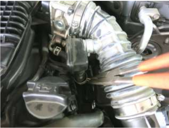
e. Disconnect the driver side PCV hose by releasing the spring clamp as shown.
