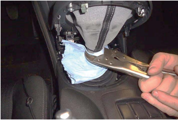
5. Hold the shift lever stationary with locking pliers. Use a rag to avoid marring the shaft.
