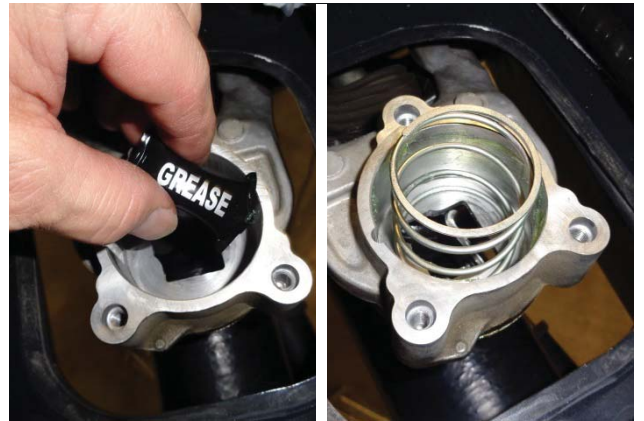
21. Apply a thin layer of grease (10) to the bottom and sides of the shifter housing. Then reinstall the spring.
