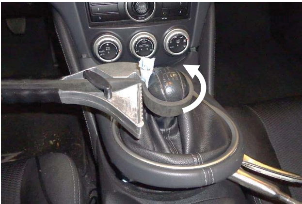
6. While holding the shift lever stationary, remove the shift knob with a strap wrench. Use a rag to avoid marring the knob.
