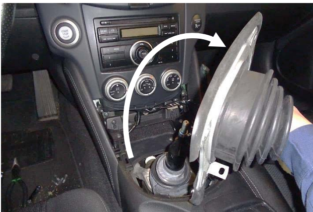
13. Lift the dust boot and metal frame off of the shift lever.
