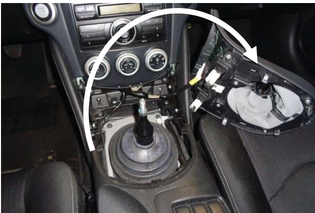
7. Carefully lift the assembled boot and shifter panel off of the shift lever.
