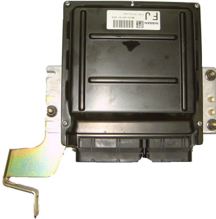
Figure 3 – OEM ECU on Mounting bracket
