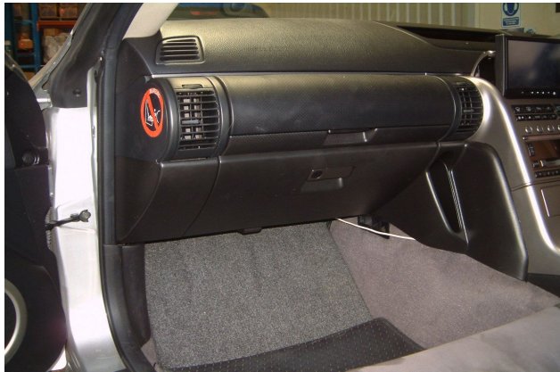
Figure 1 – ECU is located behind the glove compartment
