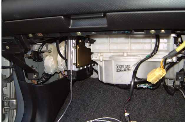
Figure 5 – Haltech ECU Installed in OEM Location
