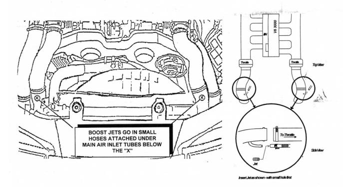
NOTE: THE BOOST JETS SUPPLIED IN THIS KIT ARE SIZED TO PRODUCE A BOOST LEVEL OF 12 TO 14 LBS. THE BOOST MUST BE CHECKED WITH AN ACCURATE GAUGE TO DETERMINE WHETHER YOUR BOOST PRESSURE IS IN THIS RANGE AFTER INSTALLING THE UPGRADE. IF BOOST IS LOWER, FULL POWER MAY BE LIMITED. IF BOOST IS TO HIGH, "PING" OR DETONATION MAY OCCUR (THIS MUST BE AVOIDED!). SPECIAL JETS CAN BE ORDERED TO CORRECT EITHER CONDITION.
